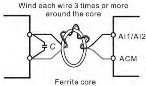
**Figure 10: Ferrite core**
