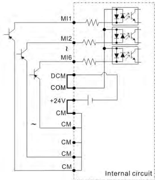
Figure 21: Source mode with internal power (+24V<sub>DC</sub>)
