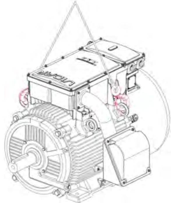
Figure 5: Example of two sling lifting
