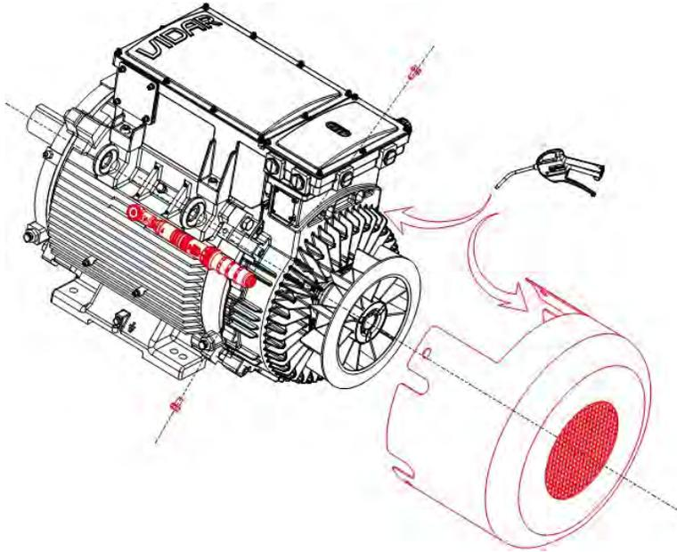
3. Use a Snap ring pliers to remove the C-clip and detach the fan backward along the axial direction.
