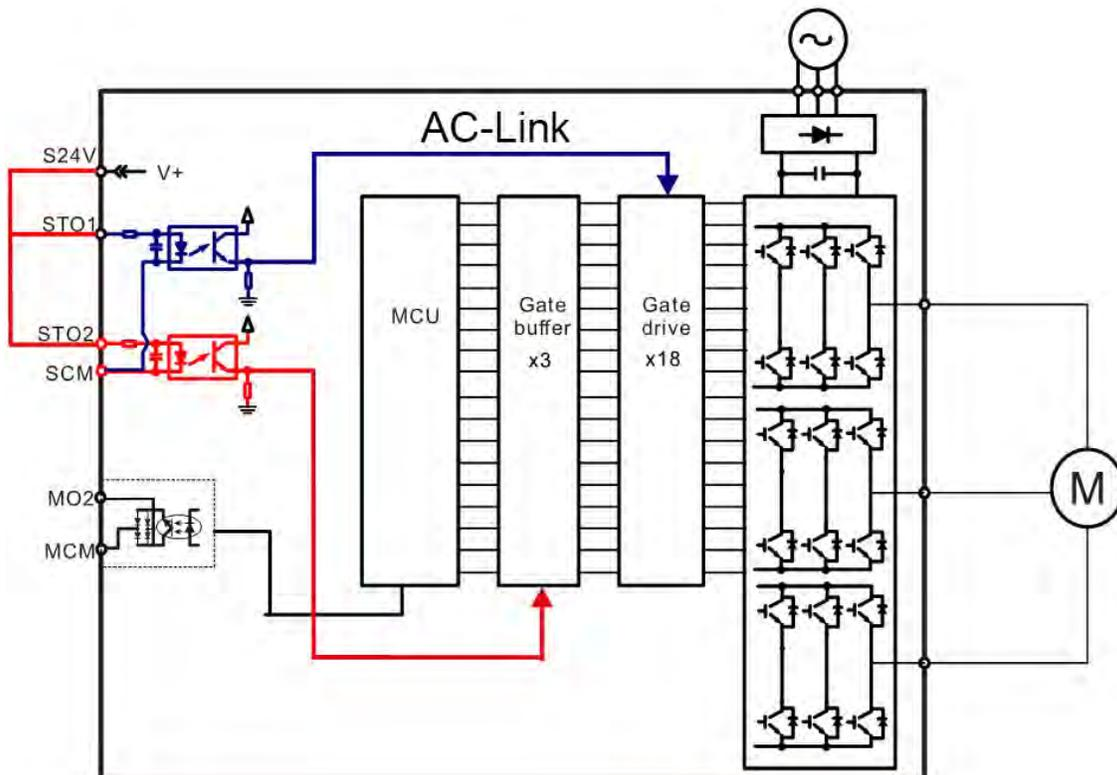
**Figure 26: Default setting for S24V-STO1-STO2 is short-circuited**
