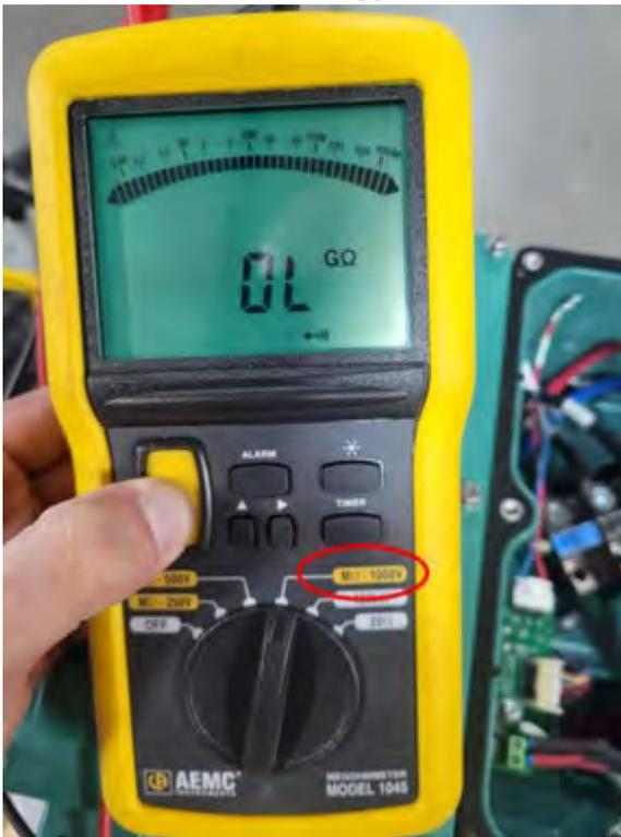
8. Hold down the yellow button until the resistance measurement no longer increases.
