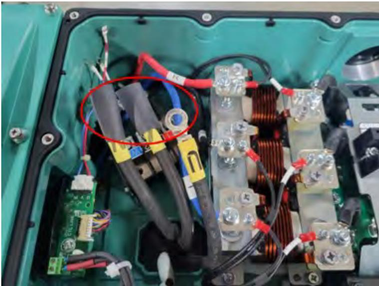
5. Attach the Megger's Black lead to a grounded connection.
