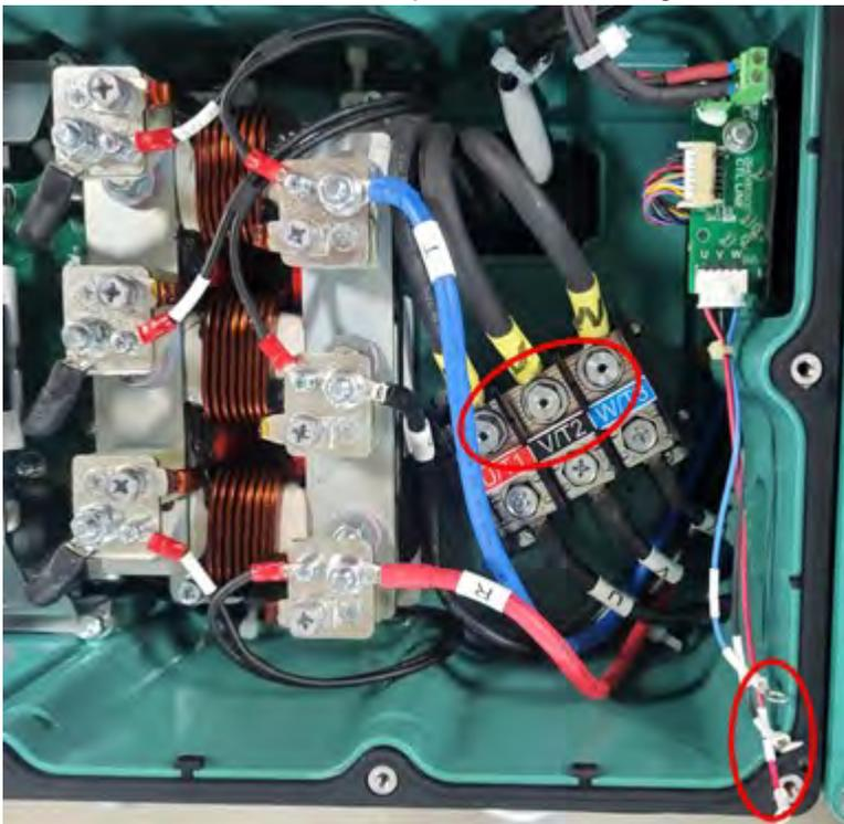
3. Disconnect all three leads: U, V, W, that supply the motor's three winding phases.
