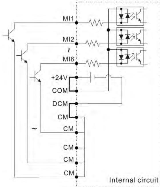
Figure 20: Sink mode with internal power (+24V<sub>DC</sub>)
