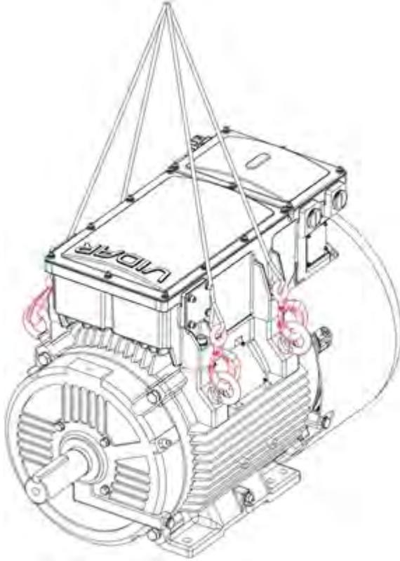
Figure 4: Example of four sling lifting
