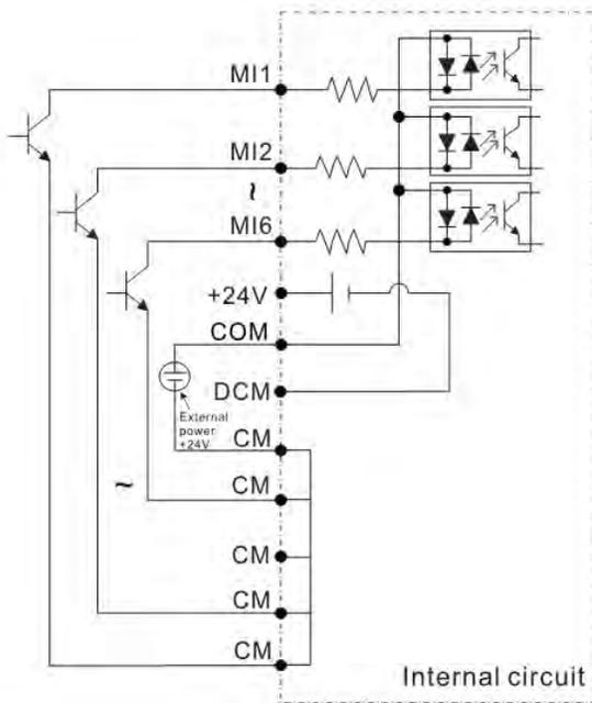
Figure 22: Sink mode with external power
