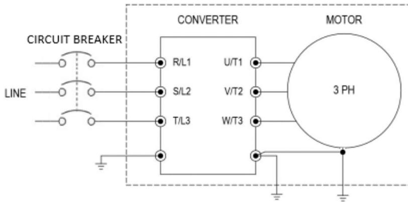
Figure 12: Main circuit terminal
