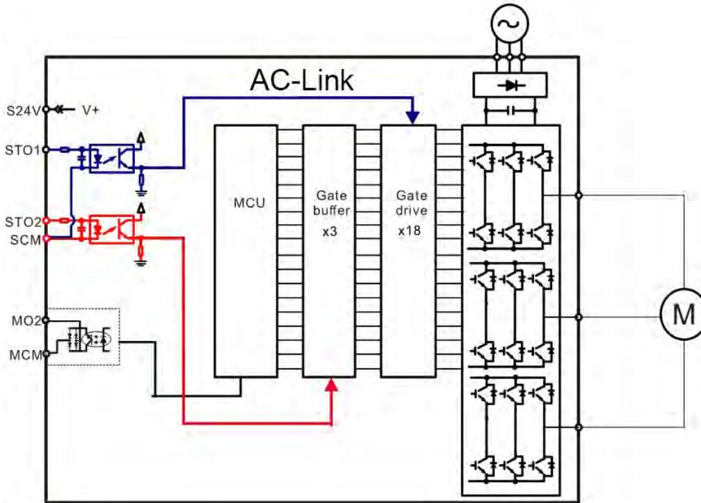
**Figure 25: Internal STO circuit**
