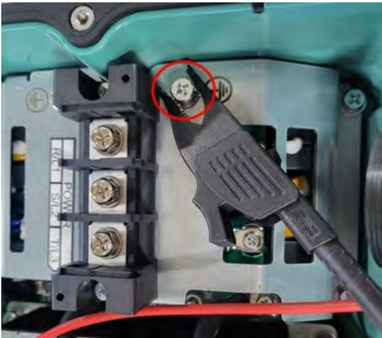
6. Attach the Megger's Red Lead to U, V or W motor phase.
