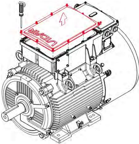
2. Remove the debris cover by pushing one side inward to release it from the grooved edge.
