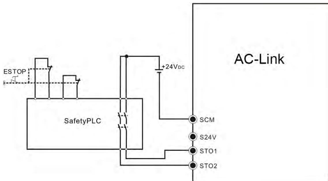
Figure 29: External 24V power wiring
