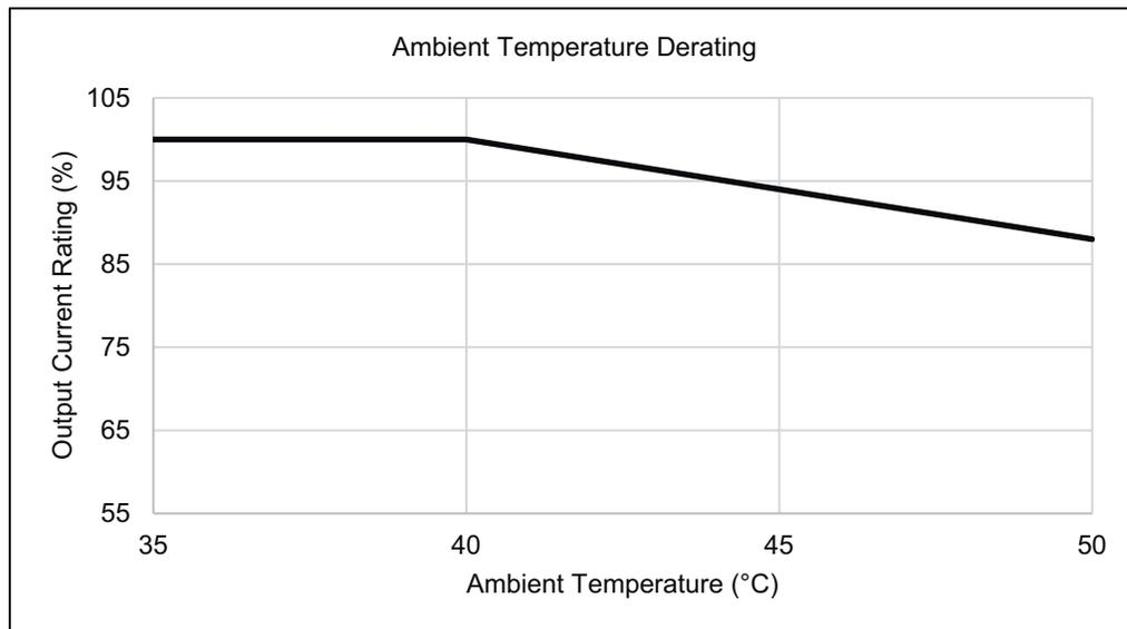
**Figure 46: Ambient temperature derating curve**
