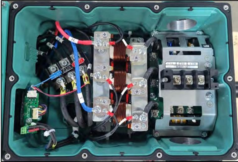
2. Unscrew and remove the three phases of the voltage sensors.
