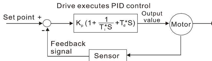
$K_p$  Proportional Gain (P),  $T_i$  Integral Time (I),  $T_d$  Differential Time (D), S Calculation
