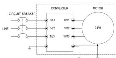
**Figure 11: Power input terminal**
