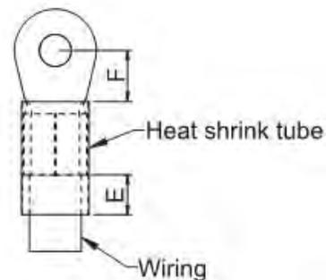
Figure 14: Heat shrink tube
