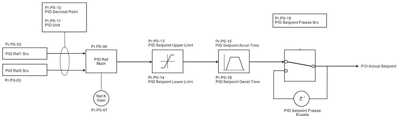
● Process PID setpoint diagram (using sleep boost function)
