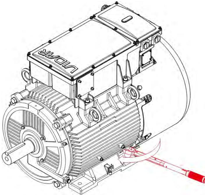
Figure 3: Example of torque wrench usage
