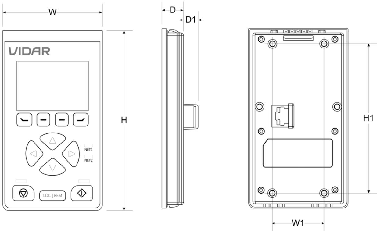
**Figure 40: Digital keypad dimensions**
