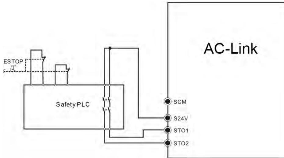
**Figure 28: Built in 24V power wiring**
