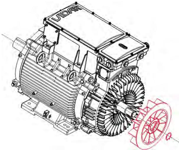
6. Put back the motor cowl and tighten back the four bolts loosened from Step 1. Refer to the table listed in Step 1 for the tightening torque.
