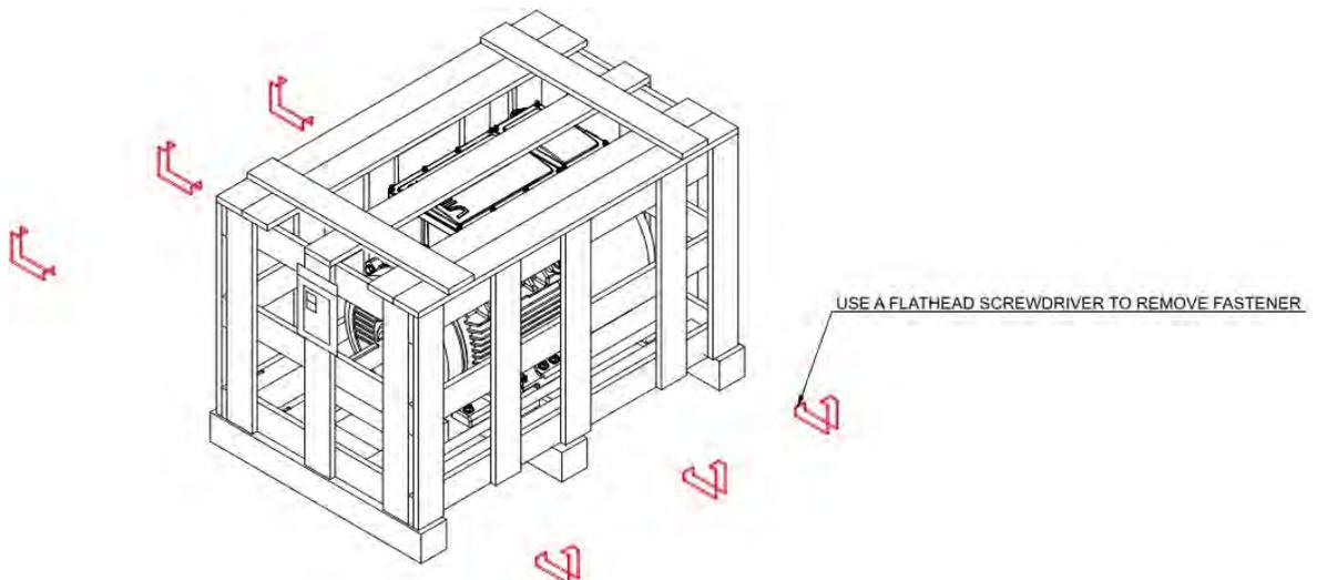
3. Open the wooden box, remove the PE bag, manual, bolts and nuts.
