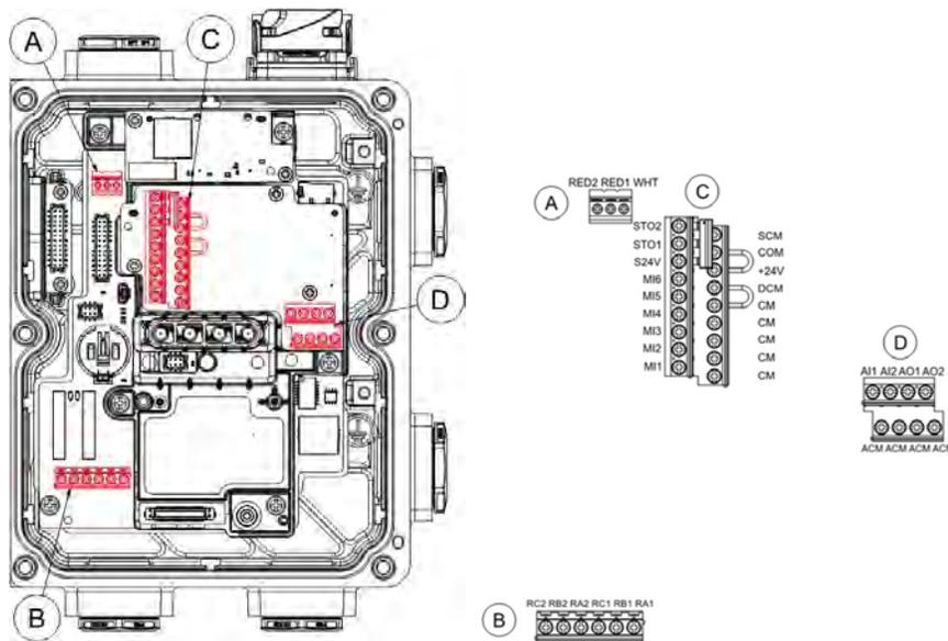
Figure 24: Terminal wiring
