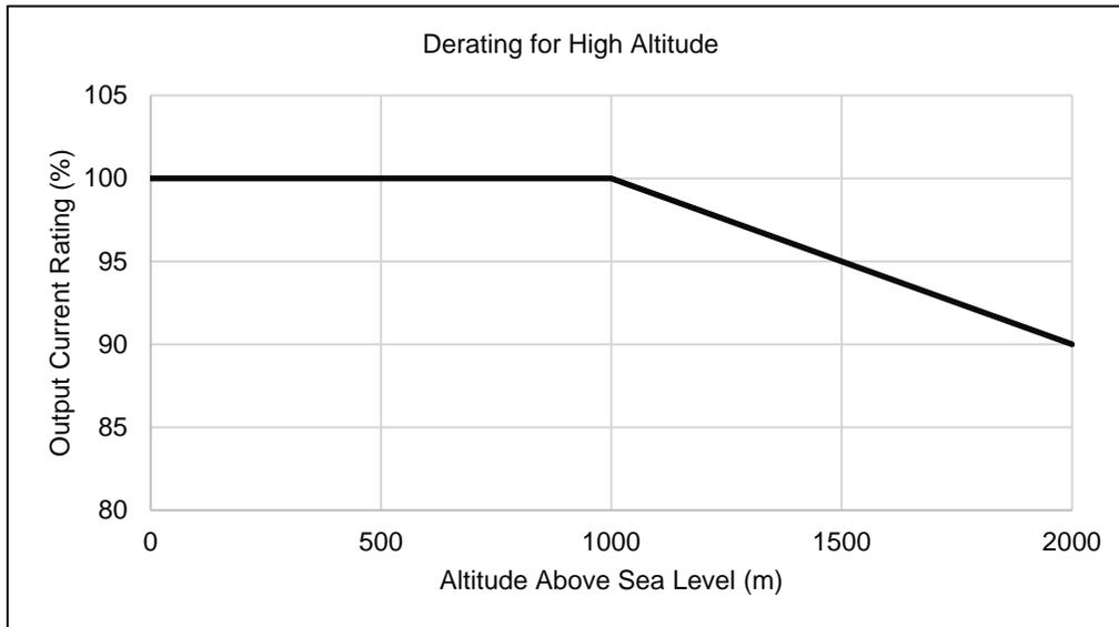
**Figure 47: Altitude derating curve**
