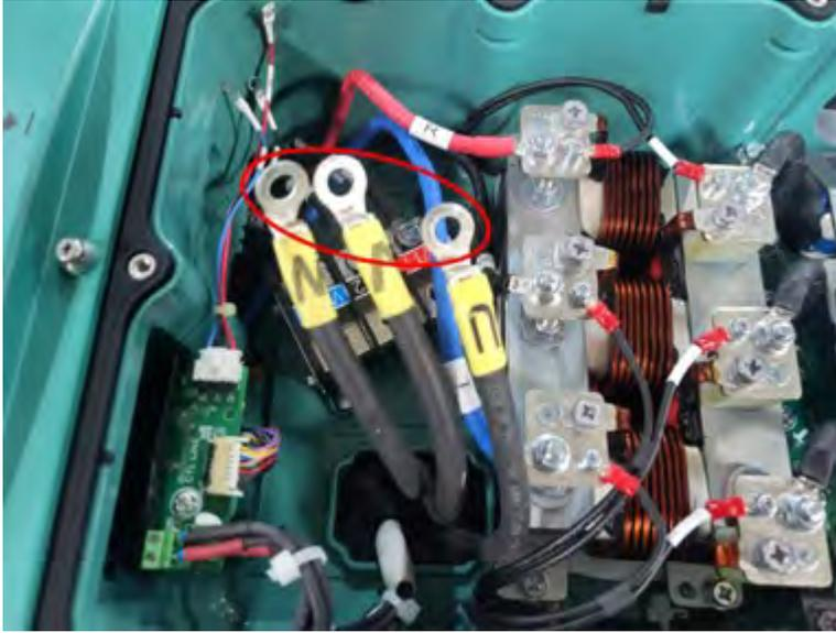
4. Isolate and insulate the motor wires to ensure they do not make contact with the motor terminal block or anything else.
