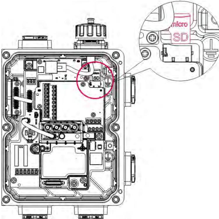
**Figure 43: SD Card installation**
