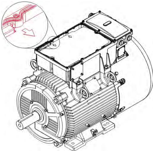
3. After the debris cover is detached from one side of the terminal box, remove the cover. Refer to [Section 4.3.3 Main circuit terminal specification on page 37](#) and [4.2 System wiring diagram on page 31](#) for further wiring information.
