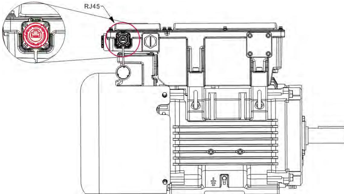
**Figure 38: Keypad connector**
