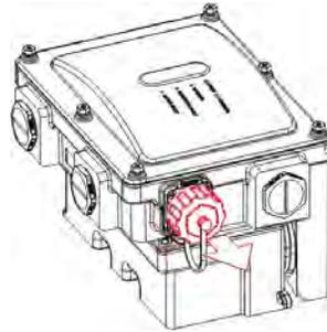
2. Install the RJ45 waterproof connector.
