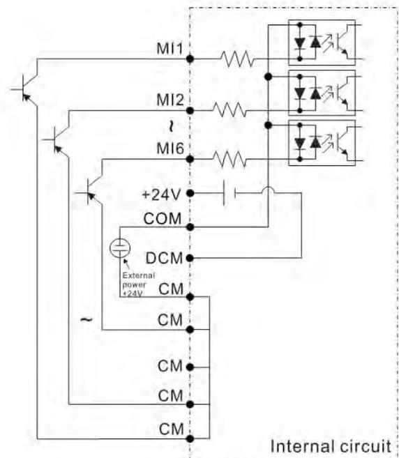
Figure 23: Source mode with external power
