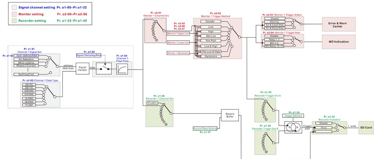
Setting process of channel selection, monitor and recorder function:
