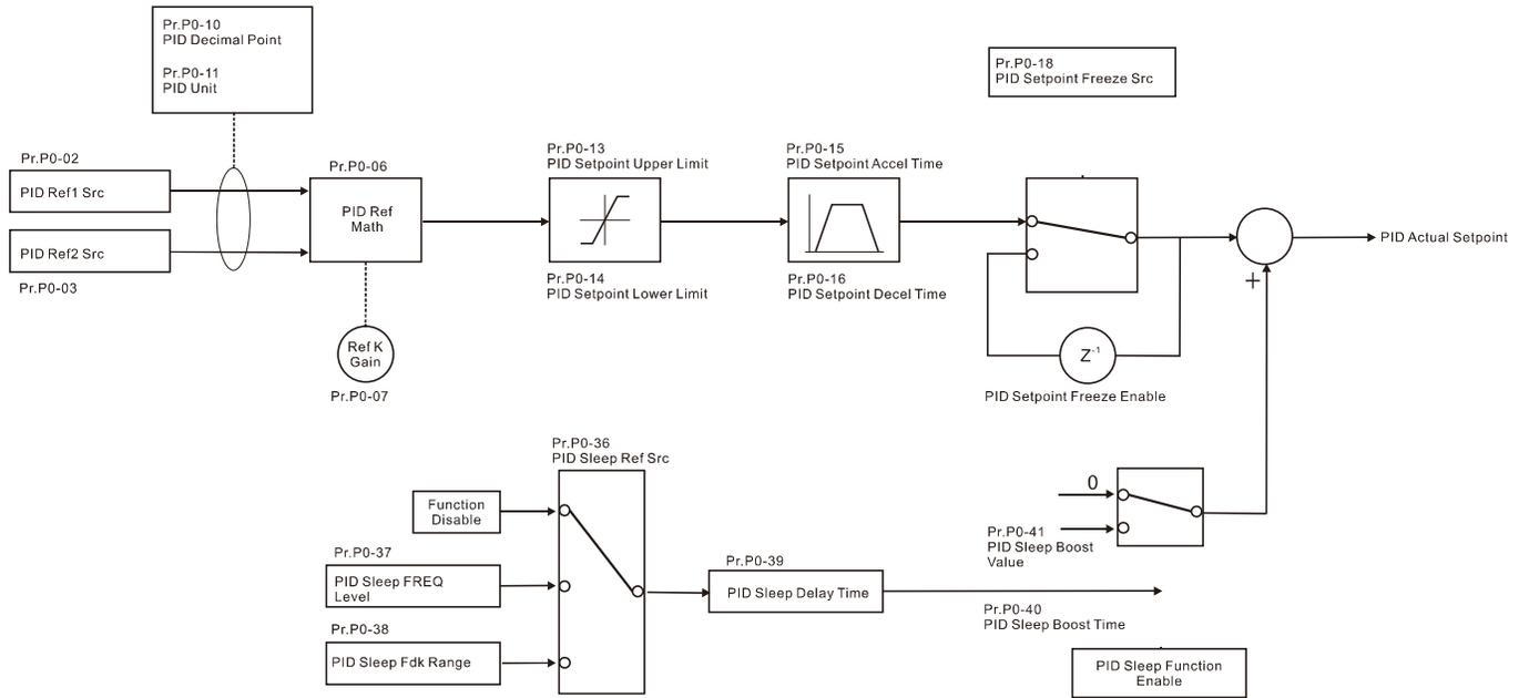
● Process PID parameter setting process.
